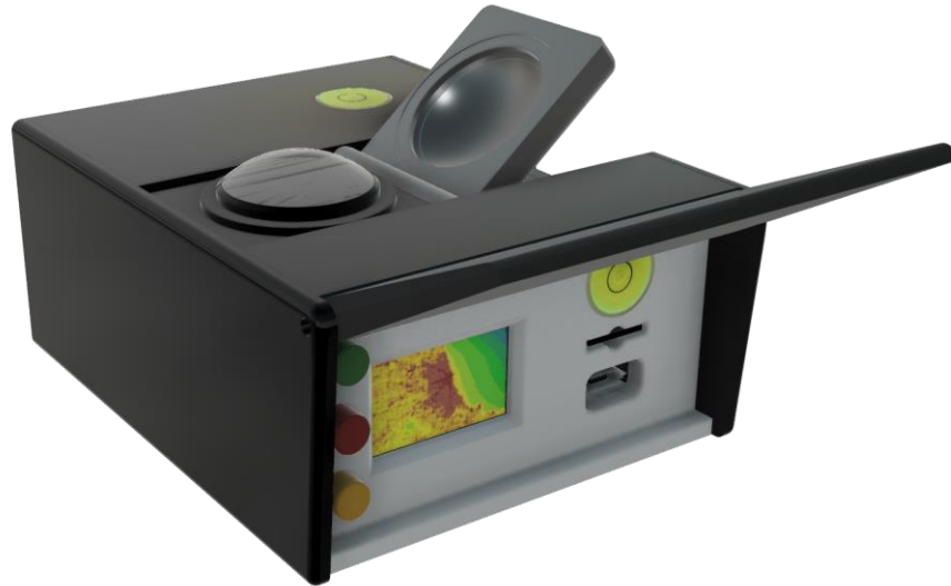
Figure 9: CAD rendering of the version 2 GONet camera in development.
