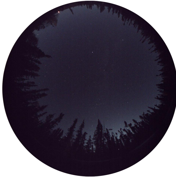
Figure 5: A stacked set of GONet images from a dark sky location (Yellowknife, Northwest Territories, Canada). Using astrometry.net, stars as faint as magnitude 4.4 were identified near the zenith.
