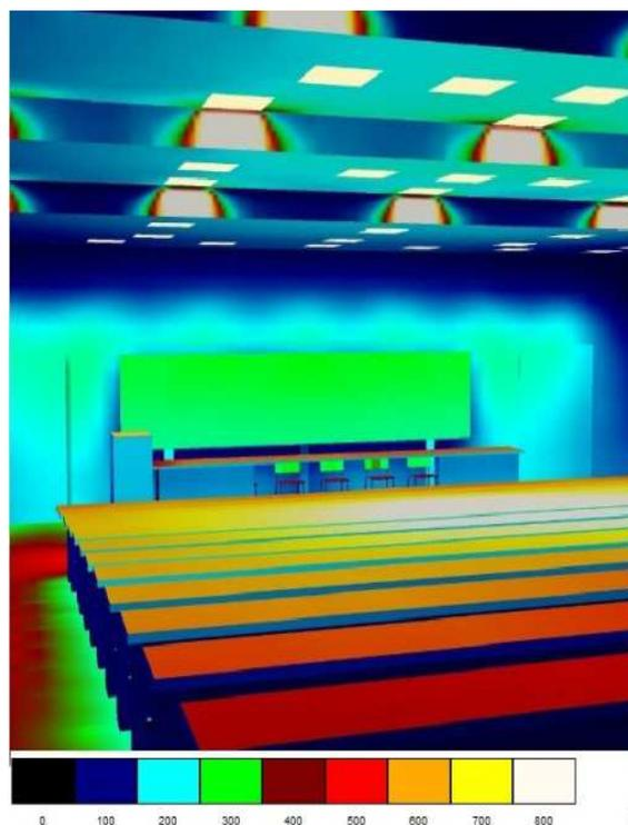
Figure 1 DIALux simulation with fluorescent lamps
