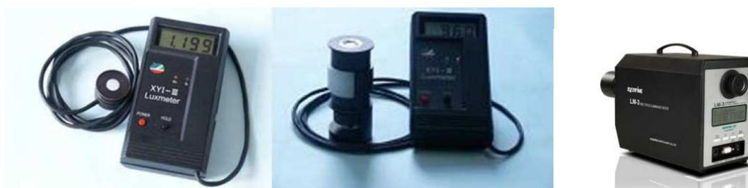
**Figure 3** Illuminance meter, semi-cylindrical illuminance meter and luminance meter used in the study.
