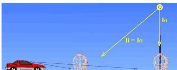
**Figure 4** Diffuse, Concrete road surface reflection characteristic
