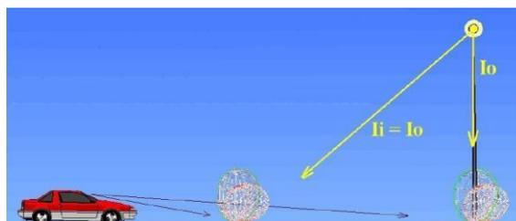
**Figure 5** Semi-diffuse, Asphaltic road surface reflection characteristic
