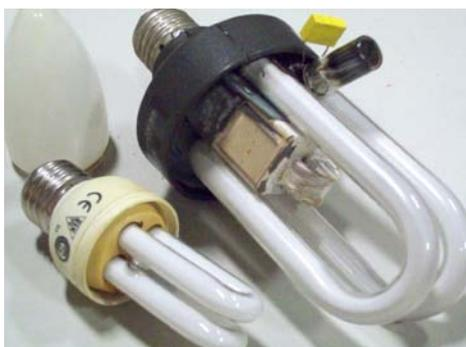
**Figure 1** Former and present technology in CFL lamps. Former lamp consisted in a mere banned fluorescent tube with conventional ballast.
