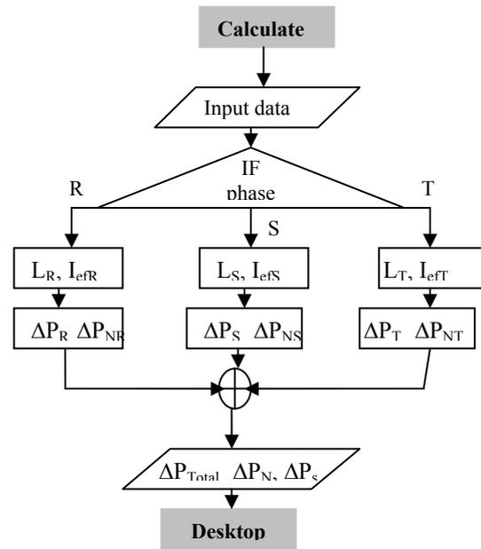
Figure 7 Working diagram of the PLM
