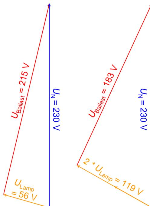
**Figure 3** Simplified vector diagram for single and tandem mode operation of a 5 W TC-S lamp – it seems that  $2*56\text{ V}=119\text{ V}$  in this case but this is because current is slightly lower in tandem mode, which makes lamp voltage greater!
