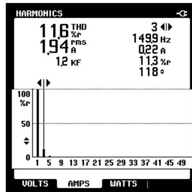
Figure 1 Harmonic current spectrum –LVF250
