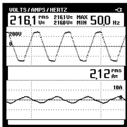
Figure 4 Voltage and current waveforms – LPN150
