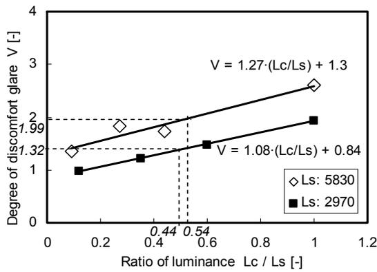
**Figure 3.** Relationship between the degree of discomfort glare and the size of the window
