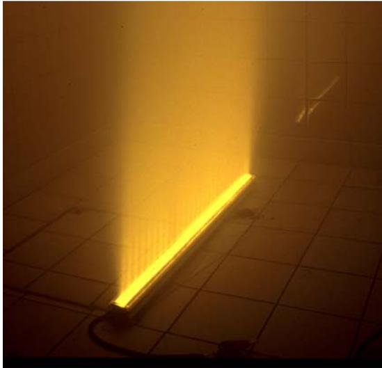
**Figure 4** Near-parallel beam of LED-line
