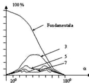
Figure 4 The output voltage harmonic content of the AC thyristor controller.
