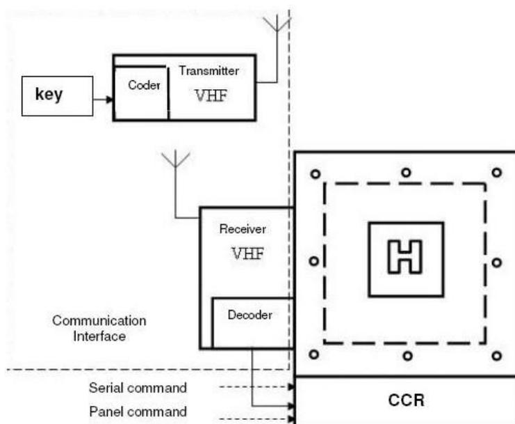
**Figure 7** Radio wireless remote control and the communication interface block diagram
