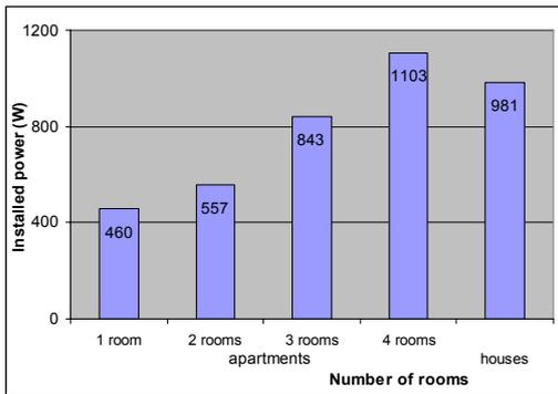
Figure 2 Average installed power in residential lighting - [9]
