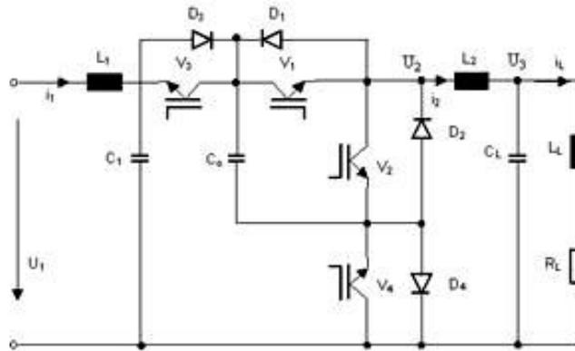
**Figure 5** The diagram of the PWM AC IGBT chopper
