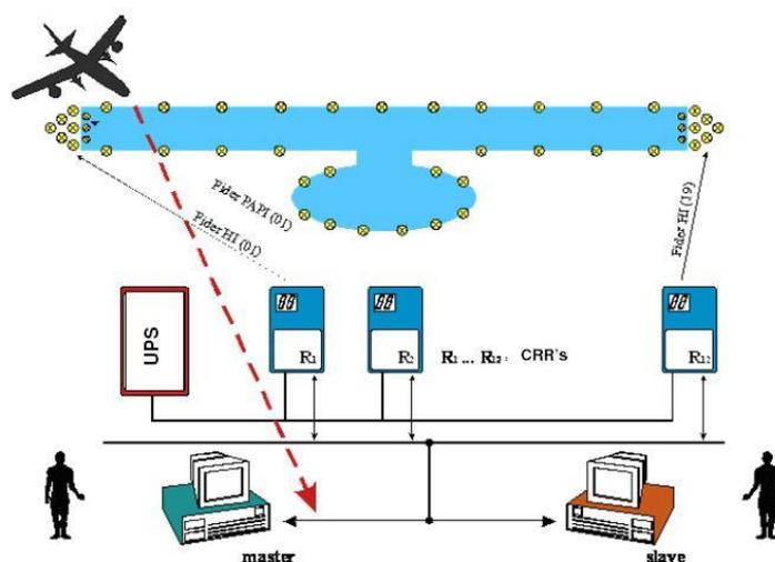
**Figure 1** Airfield lighting system block diagram with remote control units [5]
