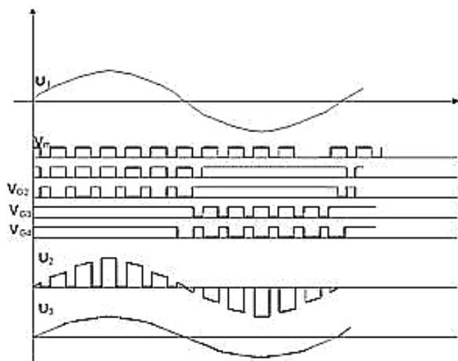
**Figure 2A2** The wave forms for the AC PWM chopper ( $V_{Gk}$  are the gate drive impulses and  $V_m$  the modulation signal)
