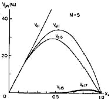
**Figure 6** Output voltage harmonic content of the PWM AC chopper
