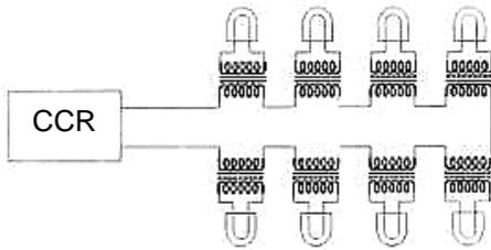
**Figure 1A1** Serial powered circuits
