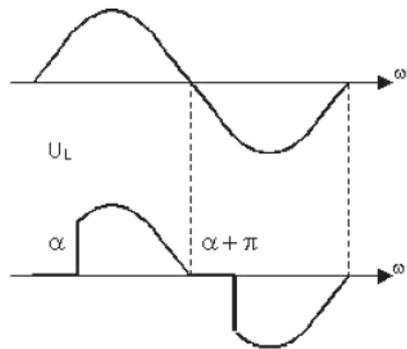
**Figure 1A2** The wave forms for the AC thyristor phase shift chopper
