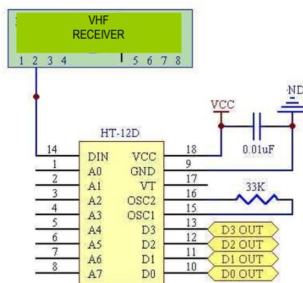
**Figure 8** The diagram of the experimented receiver decoder
