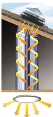
Figure 1 How the SunPipe works.
