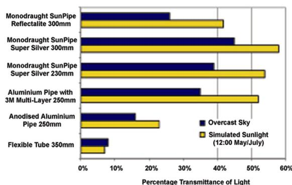
Figure 2 Results of the test on SunPipe.
