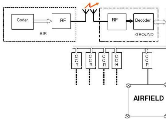
Figure 2 Airfield lighting system (heliport) block diagram with VHF wireless remote control unit [6]
