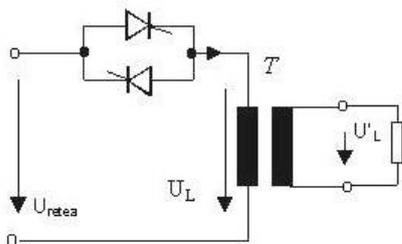
Figure 3 Diagram of the AC thyristor controller
