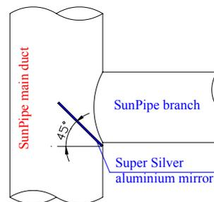
Figure 4 Mirror-supplied SunPipe branch.
