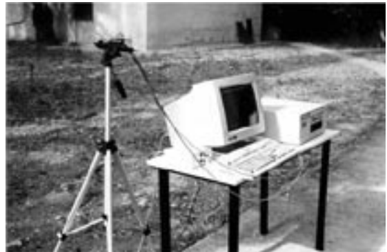
Figure 6 Passive solar radiation scanner for the determination of the atmospheric pollution
