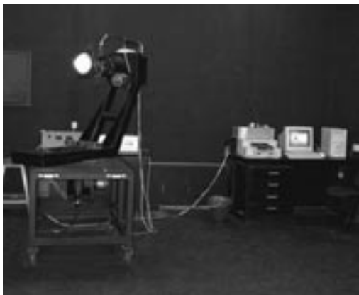
Figure 1 Goniophotometer with facility for turning the light source, CIE type 3
