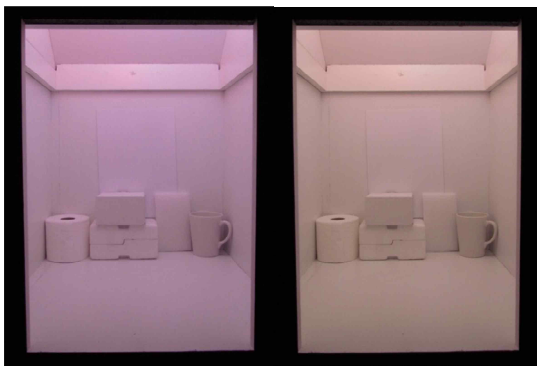
Figure 13. Test booth on the left is illuminated by a source selected by the under-40 group as yielding “white” light. It shows a higher component of blue. The test booth on the right is illuminated by a source selected by the over-50 group as yielding “white” light. It shows a smaller component of blue and a larger component of yellow.
