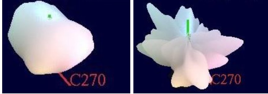
Figure 5: Spherical representation of an efficiency model taking different gloss value for optic and louvre as entries (normal to luminaire is upward). Left: optic gloss and louvre gloss are set to 0.5 and the efficiency is coherent with efficiencies in table 1. Right: optic gloss is set to 0.5 while louvre gloss is set to 1, leading to incoherent efficiency.
